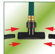
Attach connectors based on your custom layout. Hose should be inserted at least  $\frac{1}{2}$ " into the connectors to guarantee a water tight seal.
